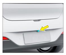
The reverse camera is located in the middle of the rear bumper, above the license plate.
