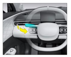
After turning on the low beam lights, push the light control lever toward the instrument panel to turn on the high beam lights, with the corresponding indicator light Dilluminating.
