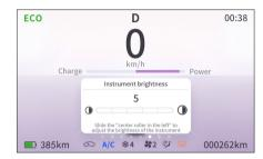
For models without MP5:Press the switch button ① to the brightness adjustment interface, and adjust the brightness using the scroll wheel ②.
