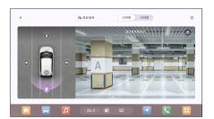
If equipped with a AVM, the driver can observe the vehicle's surroundings in all directions.
