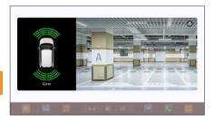
When the gear is shifted to the "R" (reverse) position, the MP5 display screen automatically switches to show the view behind the vehicle.
