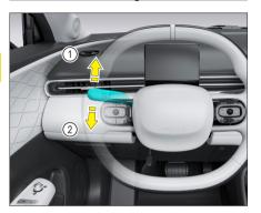
Flip the light combination switch all the way up in direction parallel to the plane of the steering wheel to turn on the right turn signal, with the right turn indicator on the instrument cluster flashing.
