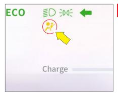
When the vehicle is powered on, the airbag system fault warning light will illuminate. If the system is functioning properly, this light will turn off after being lit for a period of time.
