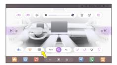
After the vehicle is powered on, press the rear window glass defogging/defrosting button on the MP5 air conditioning interface to activate rear window glass heating for defogging/defrosting, and simultaneously heat the external rearview mirror for defogging/defrosting.
