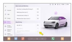
After powering up the vehicle, access MP5 Vehicle Settings—Convenient Driving screen to activate the driver's seat welcome function.
