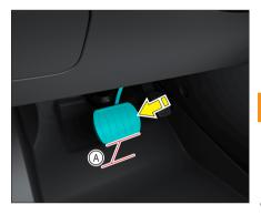
After powering up the vehicle, check the distance A between the initial position of the pedal and the carpet (A). Contact a dealership if the distance is not within the following range:
