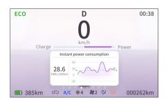
It can also switch to display instantaneous electricity consumption.
