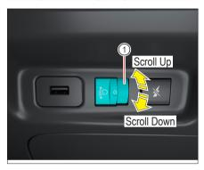
After turning on the low beam lights, the driver can rotate the manual adjustment wheel located to the left of the instrument panel to adjust the height of the headlight beam.
