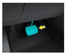
Carry the smart key, unlock and enter the vehicle, step on the brake pedal, the vehicle starts and enters READY status, and the READY indicator light on the combination instrument panel lights up.
