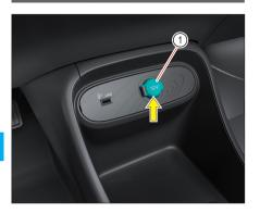
A 12V power socket 1 is located at the front of the passenger dashboard.
