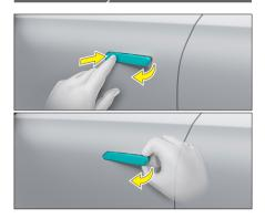
Use the mechanical key to unlock/lock the doors when the vehicle is low on power or the smart key is out of power:
