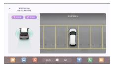
After the driver confirms the direction of parking out, touch the "Left Parking Out" or "Right Parking Out" icon on the MP5 to activate the automatic parking exit function.
