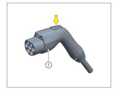
Align the charging gun and fully insert it into the AC charging port to match the charging gun with the charging base. Confirm that the charging gun is locked;
