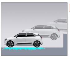
If the vehicle falls from a height and lands on its bottom, the frontal airbags may not deploy.
