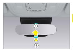
The internal rearview mirror has an antiglare feature, which reduces the glare caused by the reflection of lights from vehicles behind on the driver's eyes.
