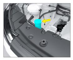
If using the windshield washer results in intermittent or no spray of washer fluid, it may indicate a lack of washer fluid. Check and, if necessary, add washer fluid to the reservoir promptly.
