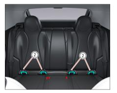
The lower anchor brackets 2 are located at the connection between the rear seat backrest and the cushion, next to the "ISOFIX" label on the cushion. Opening the reserved socket will reveal the brackets
