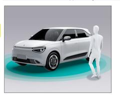
When the auto unlock feature when approaching the vehicle is enabled, carry the key and approach the vehicle (around 1.5m near the left front door handle or rear door), the doors will automatically unlock, hidden door handles automatically extend\*, and all turn signals blink twice.
