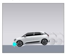
Crossing deep potholes, causing the front of the vehicle to hit the ground, may accidentally trigger the deployment of the frontal airbags.
