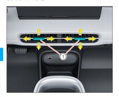
Moving control knob ① adjusts the air flow direction (up/down, left/right) of the vent to the desired position. Sliding control knob ① inward to the limit position closes the vent.
