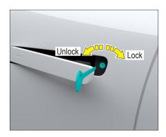
4. Turn the mechanical key toward the front/rear of the vehicle to unlock/lock the door.
