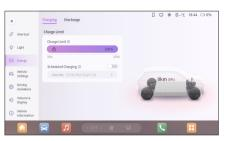
The MP5 Energy—Charging interface displays vehicle status (charging status, driving range, battery level, charging power, current, voltage, and charger connection status).
