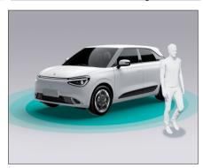
When the auto lock feature when leaving the vehicle is enabled, with the gear in P position, all doors (including the rear door) closed, carrying the key, and moving away from the vehicle (about 3m perpendicular to the left side door handle or rear door), the doors will automatically lock, hidden door handles automatically retract\*, and all turn signals blink once.
