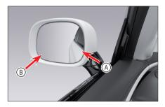
Left and right angle: The car body (A) should occupy about 1/4 of the mirror surface.
