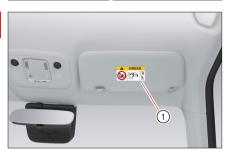
Warning instruction labels 1 are located on the surface and inside of the front passenger sun visor.
