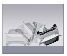
In the event of a rollover or lateral rollover accident, the frontal airbags may not deploy.
