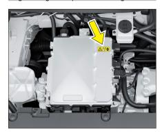
The high voltage component warning label is stuck on top of the high voltage integrated controller.
