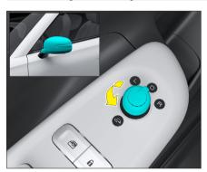
Twist the electric folding switch for the rearview mirror located on the driver's side door armrest to fold/unfold the external rearview mirror.
