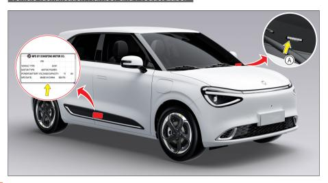
The vehicle identification code (frame number) VIN is the unique identification code of the vehicle, which can be viewed at 6 locations:
