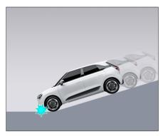
Descending steep slopes, with the front of the vehicle hitting the ground or objects like sand mounds or gravel piles, may accidentally trigger the deployment of the frontal airbags.
