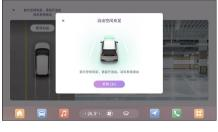
If there is insufficient space in front and behind the vehicle, the MP5 shows a prompt "Insufficient front and rear space, parking system exiting":
