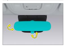
The driver can adjust the internal rearview mirror, aiding drivers of different heights in observing the rear of the vehicle at any time, thus enhancing driving safety.
