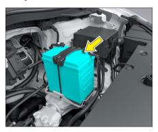
When replacing the 12V battery, ensure that it is correctly installed and securely fastened.
