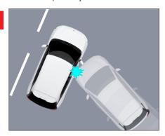
When the vehicle's side cabin area is impacted, the frontal airbags generally will not deploy.
