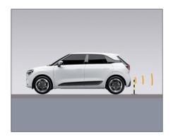
Thin or slender objects like steel cables, chains, thin poles, and stakes might not be detected.
