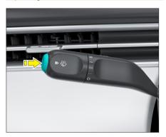
Hold down the front windshield wash button, the front nozzles start spraying the washer fluid, then the front wipers begin to wipe.
