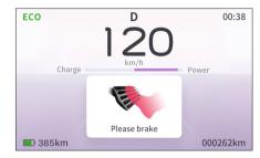
When there is a collision risk ahead, the vehicle will issue an urgent warning, the combination instrument indicator light flashes with a pop-up "Please press the brake pedal," accompanied by a buzzer sound alarm reminder.
