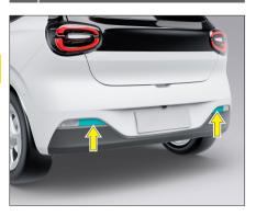
The Response Reflector is designed to reflect the lights of vehicles from behind, reminding the drivers of the trailing vehicles to maintain a safe driving distance.
