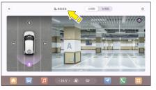
Turn on the READY light, enter the surroundview interface from the quick menu bar, press the automatic parking assist button, shift to D gear, and start the automatic parking feature. The vehicle automatically enters the parking space search interface.
