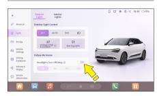
After the vehicle is powered down during night-time parking lock, the Follow Me Home feature can be activated. The headlights automatically turn on and delay turning off, illuminating your way home.
