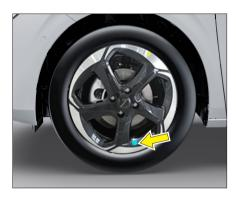
Remove the valve cap from the tire valve stem and check for air leaks using the soap solution method.
