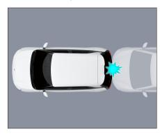
When the vehicle is only rear-ended or impacted from the rear, the frontal airbags will not deploy.
