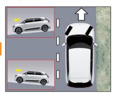
Turn the wheels to the side of the road to prevent the vehicle from moving towards the center of the road.
