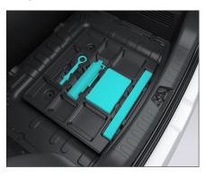
The onboard tools are stored under the foam pad beneath the trunk floor and fixed behind the rear panel. They can be accessed by lifting the trunk floor.
