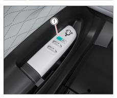
Press the switch 1 to disable the function of all passenger window controls; however, the driver's side window switch can still operate to raise and lower the window.
