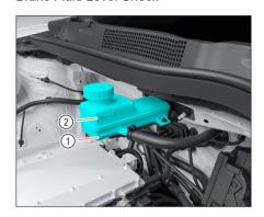
Check the fluid level in the reservoir. If the brake fluid level is below the MIN line ①, the brake system warning light will illuminate. Add brake fluid up to the MAX line ②.
