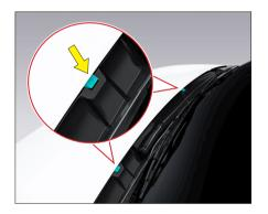
If there is debris near the washer nozzle, clean it promptly as it may affect the normal functioning of the windshield washer.
