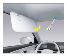
Detach the sun visor from the central support ② and turn it to the side to block glaring light coming from the side.
