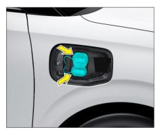
Remove the dust cover to reveal the charging ports.
