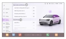
In the Vehicle Settings→Door Locks and Windows Options Bar ①, you can control the door lock and window functions: Auto Door Locking When Driving Switch, Walk Away Auto Lock\* Switch, Proximity Auto-Unlock\* Switch, Windows Auto-Up on Lock Switch.
