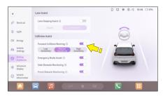
The Forward Collision Warning Assistance can be turned on/off in the MP5 assisted driving → collision assistance interface. The sensitivity of the warning (low, medium, high) can also be set.
