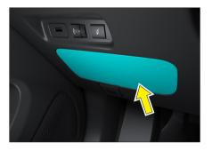
The cabin fuse box can be accessed by removing the cover panel located on the lower left side of the dashboard.
