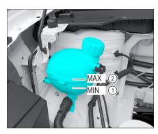
Check the coolant level after the radiator has cooled.
