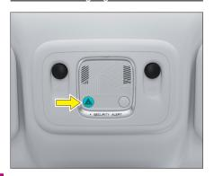
The hazard warning light switch is located on the front overhead light switch panel. In emergency situations, use the hazard warning lights to alert other road users, helping to avoid traffic accidents.
