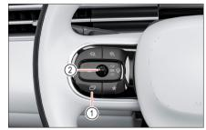
Press the instrument function switch button 1 on the left side of the multifunction steering wheel to switch the display of card information on the instrument panel. Some functions can be adjusted via Settings 2.
