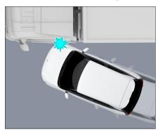
When the vehicle collides with road guardrails or other vehicles from a front-side angle, the frontal airbags may not deploy.
