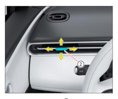
Moving control knob 2 adjusts the air flow direction (up/down, left/right) of the vent to the desired position. Sliding control knob 2 inward to the limit position closes the vent.
