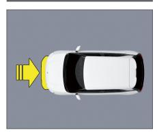
In the event of a collision, the system controls whether the frontal airbags inflate based on the angle and intensity of the impact detected by the collision sensors within the vehicle monitoring area (as shown above).
