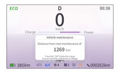
Vehicle maintenance reminder information is also displayed. When the distance to maintenance is less than 500km, a popup will display "Distance from next maintenance of XXX km" every time the vehicle is powered on.
