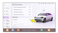
Under certain conditions (the vehicle starts in sand, snow or soft road), the convenient driving interface on MP5 vehicle can be set, and the ESC function is turned off, and the ESC turnoff indicator light on the instrument cluster can be set
