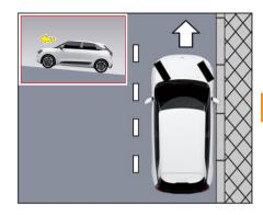
Turn the steering wheel away from the curb and move the vehicle backward until the wheel on the curb side touches the curb gently.
