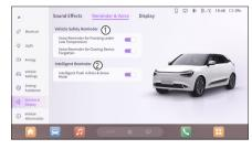
In the Volume & Display→Reminder & Voice→Vehicle Safety Reminder Options Bar ① , you can set the following alert sounds: Seat Belt Not Fastened Alert Sound, and Low Temperature Frost Alert Sound.
