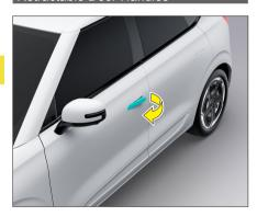
The vehicle is equipped with retractable door handles to reduce aerodynamic drag, providing a better driving experience.
