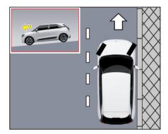
Turn the steering wheel in the direction of the curb and let the vehicle forward until the wheels on the curbside touch the curb gently.
