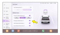
The Emergency Collision Assistance function can be turned on/off in the MP5 assisted driving  $\rightarrow$  collision assistance interface.
