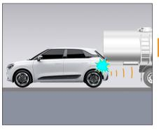
Obstacles above the detection range, like hanging items, partially open rolling shutters, or the rear of trucks, might not be detected.
