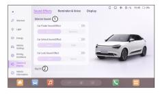
In the Volume & Display→Sound Effects interface→Exterior Sound Options Bar ① , you can set exterior sounds: Car Unlock Sound Effect, Car Lock Sound Effect,.
