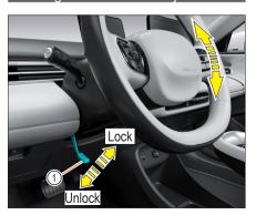
Release the steering wheel adjustment lock handle 1 downward to unlock the steering wheel, allowing adjustment of the steering wheel's up and down positions for the comfort and safety of drivers of different statures
