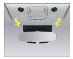
The microwave window is located around the rearview mirror in the car, and communication equipment, such as ETC, access control, intelligent parking and other equipment, can be installed in this area. Solar film is not allowed in this area to ensure the effective reading of data.
