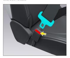
Press the red button on the buckle to release the seat belt lock. After unlocking, push the seat belt slightly towards the upper anchor point, and it will automatically retract into the retractor.
