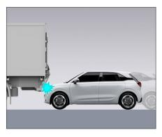
When involved in a rear-end collision with a large truck and going under the vehicle, the frontal airbags may not deploy.
