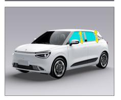
After the vehicle is powered down, holding the lock/unlock button on the smart key can control the automatic raising/lowering of the windows.
