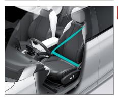
The seat belt should be placed over the body's skeletal structure. For the upper body, the upper part of the seat belt should fit snugly across the chest and over the shoulder. For the lower body, the lower part of the seat belt should fit snugly over the pelvic bones, and not rest on the abdomen.
