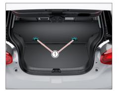
This vehicle is equipped with 2 sets of ISOFIX child seat fixation devices, each including 1 upper anchor bracket ① and two lower anchor brackets ② .
