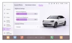
For models with MP5:Adjust the instrument panel brightness in the MP5 Volume & Display  $\rightarrow$  Display interface.
