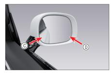
Left and right angle:The car body © should occupy about 1/4 of the mirror surface.
