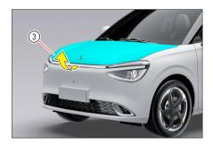
3. Lift the powertrain compartment lid 3 upwards.
