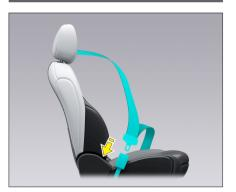
During emergency braking or a collision, the seat belt restrains the driver and passengers on their seats, preventing secondary collisions with other parts inside the vehicle, while also ensuring optimal protection from the airbags.
