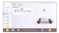
In the Energy  $\rightarrow$  Discharging interface  $\rightarrow$  Discharge Limit Options Bar, slide ① left and right to set the discharge limit, with an adjustment range of 20% to 50%. When the battery reaches the limit, a pop-up will prompt "Remaining battery has reached the discharge limit, stop discharging".
