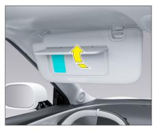
Only the driver's side vanity mirror is equipped with an LED soft light. The light turns on when the sun visor is opened and off when the visor is closed.
