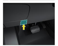
The vehicle is equipped with a Diagnostic Interface (OBD) located at the lower left side of the dashboard. It is used for digital communication between the vehicle's electronic control unit and diagnostic equipment. Connecting devices such as diagnostic tools to this interface can access vehicle electronic control unit data, fault codes, VIN, and other information.
