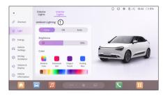
In the Lights  $\rightarrow$  Interior Lights interface  $\rightarrow$  Ambient Light Options Bar 1, you can set the ambient lights: Close, ON, and Auto. You can also adjust the brightness of the ambient light and set the color of the ambient light.
