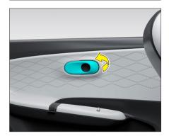
When the car door is locked, you need to pull the interior door handle once to unlock that door, and then pull it again to open the door. This prevents the accidental opening of the door while driving.
