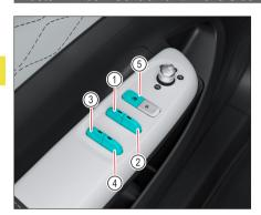
The master power window switch on the driver's side door armrest can control the raising and lowering of all window glasses and disable the passenger window control switches.
