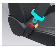
Slowly pull out the seat belt from the retractor, then insert the tongue into the buckle until you hear a "click" sound. Pull back on the seat belt to ensure it is securely locked.
