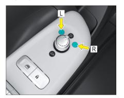
The adjustment device is located on the driver's door armrest.
