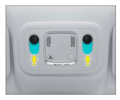
Touch the switch for the front overhead light to turn on or off the corresponding side light.
