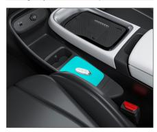
When the smart key battery is low, place the smart key in the emergency start area (as shown) with all doors closed, depress the brake pedal to start the vehicle in an emergency.
