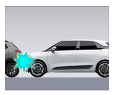
In the event of a rear-end collision with a vehicle moving in the same direction, the frontal airbags may not deploy.
