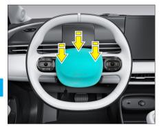
Pressing and holding any one of the three positions shown in the illustration will activate the horn.Releasing the horn switch will stop the horn from sounding.
