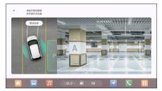
5. After selecting a parking spot, the MP5 display will show "Please release the brake pedal and remove your hands from the steering wheel." Once the driver confirms that the surrounding environment is safe, they should release the brake pedal and remove their hands from the steering wheel, and the system will begin to automatically park the vehicle into the space.
