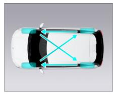
Rotate the wheels diagonally during wheel rotation.
