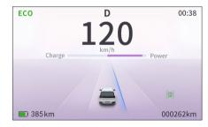
line, at risk of deviating from the lane, and without using the turn signal, the respective intervention side lane line turns blue.
