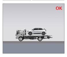
It's recommended to use a flatbed tow truck as the primary method, where the vehicle is directly loaded onto the rescue vehicle. This is the best method for transporting a vehicle.
