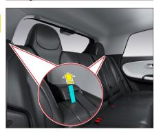
The rear seat can be folded down entirely to expand the trunk's volume.
