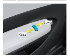
Passenger side window controls allow for the operation of the corresponding side window.
