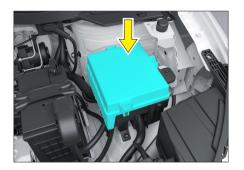
The powertrain compartment fuse box is located next to the 12V battery. Opening the fuse box cover will reveal the fuses.
