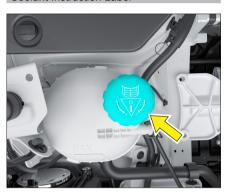
The coolant instruction label is engraved on the cap of the drive motor coolant reservoir.
