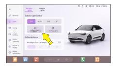
This function can be turned on/off in the MP5 lighting  $\rightarrow$  external lights  $\rightarrow$  external light control interface.
