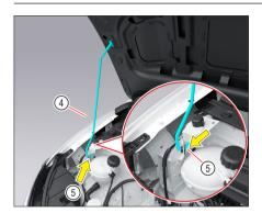
Stabilize the powertrain compartment lid and insert the support rod 4 into the support hole 5.
