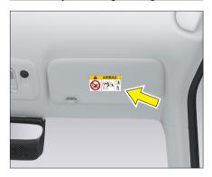
Child safety and airbag warning instruction labels are located on the surface and inside of the front passenger sun visor.
