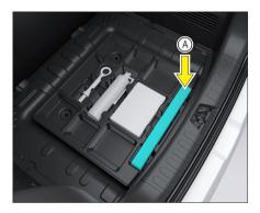
The triangular warning sign is stored under the foam pad A beneath the trunk floor A.Lift the trunk floor handle and open the trunk floor to access it.
