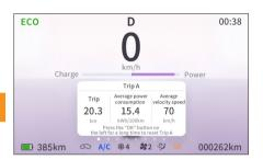
Pressing the switch button toggles between Trip A and Trip B subtotal information, displaying subtotal mileage, average electricity consumption, and average speed.
