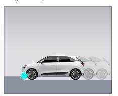
Hitting raised objects or curbs on the roadside, or severe scraping of the undercarriage with road protrusions, may accidentally trigger the deployment of the frontal airbags.
