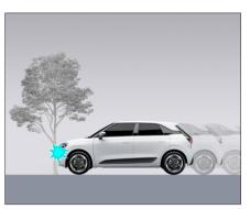
If the vehicle collides with thinner or less rigid pole-like objects such as electric poles or trees, the frontal airbags may not deploy.
