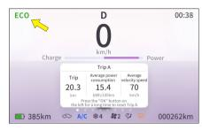
The driving mode can be viewed in the upper left corner of the combination instrument panel.
