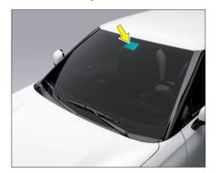
Upon vehicle power-up, the combination light switch defaults to the automatic light position, and the automatic headlight ON indicator illuminates. When the external light is insufficient, the position lights and low beam lights will automatically turn on, with the position light and low beam light indicators illuminating on the instrument cluster.
