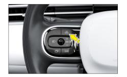
Models without MP5:Press the driving mode button on the left side of the multifunction steering wheel to switch driving modes.There are three modes:Economy mode, Comfort mode, Sport mode.
