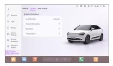
In the Vehicle Information→System interface→System Information Options Bar, you can query system information: Serial Number, Version Information, Disclaimer, and Factory Reset.
