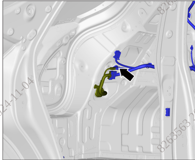
Rear Bumper Harness IC90BF Connects to Body Harness IC90BM
