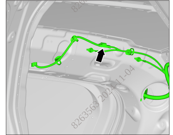
Tailgate Auxiliary Harness IC80CM Connects to High-Mounted Stop Light Harness IC80CF
