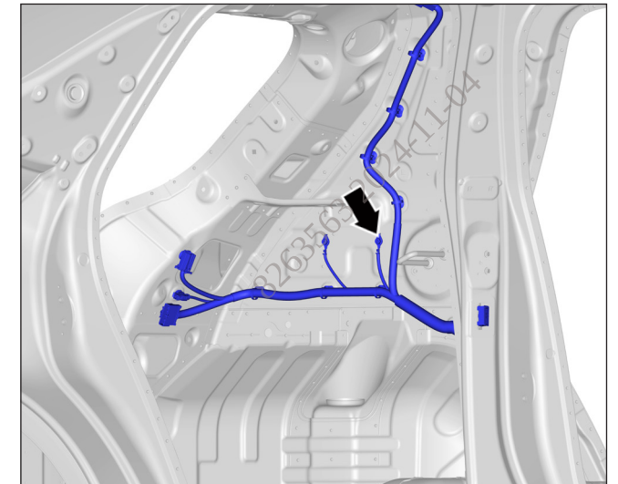
GP207 Grounding Point: Installed on the left rear wheel arch, arrow indicates position.
